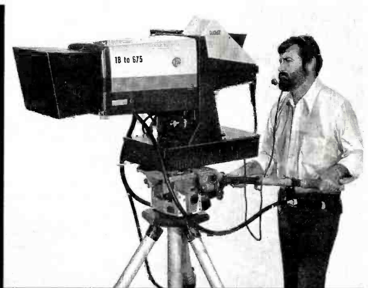
Studio camera conversion using Minimax adaptor.
